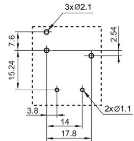
Remark: 1) In case of no tolerance shown in outline dimension: outline dimension  $\leq 1\text{mm}$ , tolerance should be  $\pm 0.2\text{mm}$ ; outline dimension  $> 1\text{mm}$  and  $\leq 5\text{mm}$ , tolerance should be  $\pm 0.3\text{mm}$ ; outline dimension  $> 5\text{mm}$ , tolerance should be  $\pm 0.4\text{mm}$ .
