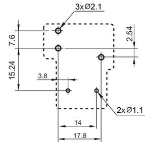
Remark: 1) In case of no tolerance shown in outline dimension: outline dimension  $\leq 1$ mm, tolerance should be  $\pm 0.2$ mm; outline dimension  $> 1$ mm and  $\leq 5$ mm, tolerance should be  $\pm 0.3$ mm; outline dimension  $> 5$ mm, tolerance should be  $\pm 0.4$ mm.
