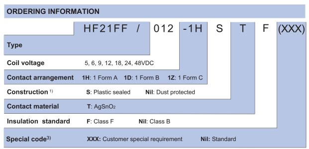
Notes: 1) Under the ambience with dangerous gas like H<sub>2</sub>S, SO<sub>2</sub> or NO<sub>2</sub>, plastic sealed type is recommended; Please test the relay in real applications. If the ambience allows, dust protected type is preferentially recommended.
