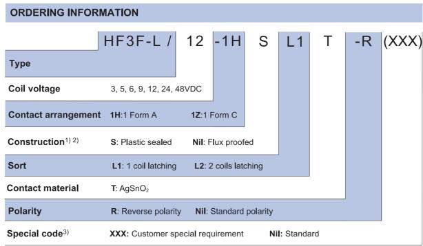
Notes: 1) We recommend flux proofed types for a clean environment (free from contaminations like  $H_2S$ ,  $SO_2$ ,  $NO_2$ , dust, etc.) . We suggest to choose plastic sealed types and validate it in real application for an unclean environment (with contaminations like  $H_2S$ ,  $SO_2$ ,  $NO_2$ , dust, etc.)
