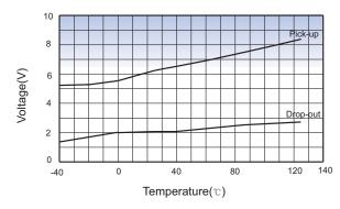
Notes: When the coil voltage is at 12V, the data above is taken as sample value and only for reference (Sample quantity: n=3)
