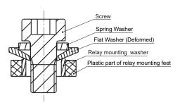
When use M5 screw, the thickness and strength of the washer needs to be guaranteed or it may stand deformation and burst the cover.
