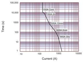
Notes: The data above is measured at the environment temperature 85°C with cross section area of wire ≥50mm². This data is only for reference and please do not use it for fuse selection.
