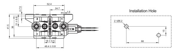
Remark: In case of no tolerance shown in outline dimension: outline dimension  $\leq$ 10mm, tolerance should be  $\pm$ 0.3mm; outline dimension >10mm and  $\leq$ 50mm, tolerance should be  $\pm$ 0.5mm; outline dimension >50mm, tolerance should be  $\pm$ 0.8mm.
