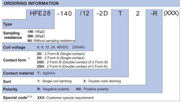
Notes: 1) 2H, 2SH means that relay is on the "reset" status when delivery; 2D, 2SD means that relay is on the "set" status when delivery. If no speical required by customer, we will keep the relay on the "set" status when delivery
