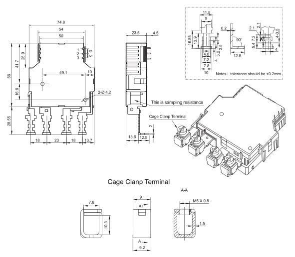
Remark: In case of no tolerance shown in outline dimension: outline dimension ≤1mm, tolerance should be ±0.2mm; outline dimension >1mm and ≤5mm, tolerance should be ±0.3mm; outline dimension >5mm, tolerance should be ±0.4mm.
