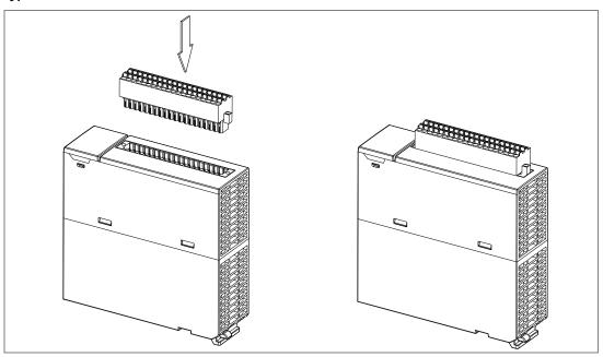
2. Press the clip in the direction indicated by the arrow. For high-definition terminals(Type 2), a flat head screw driver is required to fasten the screws on both ends.
