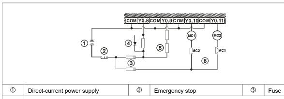
The output terminals of a transistor module are open-collector output terminals. If Y0.8 is a pulse train output terminal of a transistor module, the output current passing through its output pull-up resistor must be greater than 0.1 A to ensure that the transistor module operates normally.
