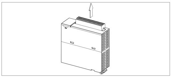
3. The terminal block is removed.
