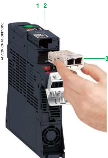
Example of installing a communication module 3 (view of underside)
