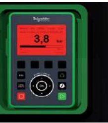
Detected fault: The screen's red backlight is activated automatically
