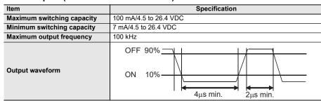
Note: 1. The load for the above values is assumed to be the resistance load, and does not take into account the impedance for the connecting cable to the load.
