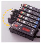
If the FS-V1 digital calibration fiberoptic sensor is configured as the main unit with several expansion units connected to it, the light quantity and sensitivity of the expansion units can be checked on the FS-V1's monitor. While viewing the monitor, the sensitivity of the expansion units can be finely adjusted.
