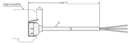
\* E3X-CN11: 4 dia. cable / 3 conductors / Standard length: 2 m (Conductor cross section: 0.2 mm² (AWG24), Insulator diameter: 1.1 mm)
