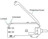
Note: To maintain the fiber unit properties, confirm that the lock is released before removing the fiber unit.
