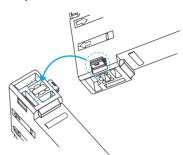
2. Remove the clip by rotating the Amplifier Unit.
