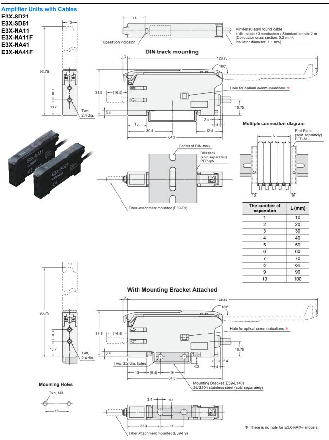
Note: When using E39-L143 Mounting Brackets, there will be small gaps between the Fiber Amplifier Units if they are mounted side by side.
