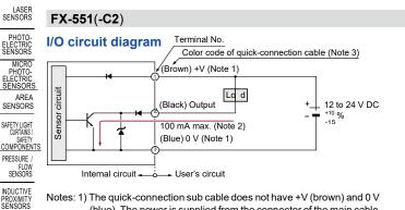
Notes: 1) The quick-connection sub cable does not have +V (brown) and 0 V (blue). The power is supplied from the connector of the main cable. 2) 50 mA max., if five amplifiers or more, are connected together. 3) The color code of the connector attached cable is also the same.
