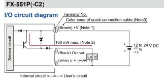
Notes: 1) The guick-connection sub cable does not have +V (brown) and 0 V (blue). The power is supplied from the connector of the main cable. 2) 50 mA max., if five amplifiers or more, are connected together. 3) The color code of the connector attached cable is also the same
