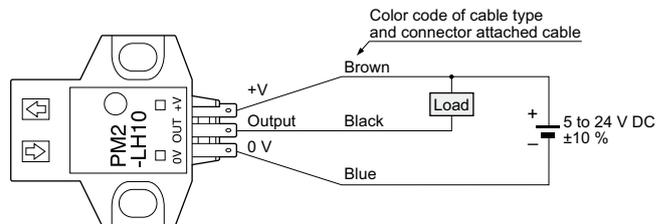
Note: Make sure to connect terminals correctly as the sensor does not incorporate a reverse polarity protection circuit.
