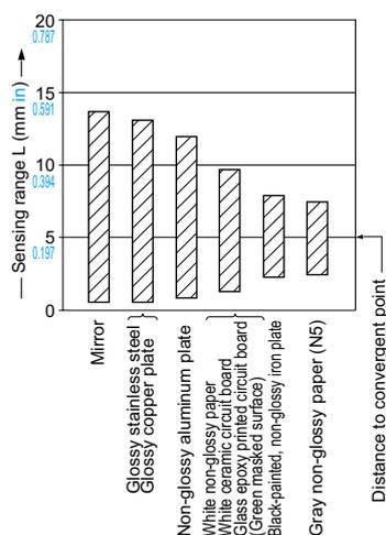
The bars in the graph indicate the sensing range (typical) for the respective material. However, there is a slight variation in the sensing range depending on the product. Further, if there is a reflective object (conveyor, etc.) in the background of the sensing object, since it affects the sensing, separate it by more than twice the sensing range shown in the left graph.
