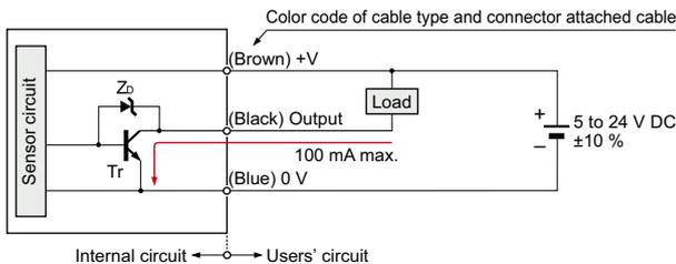
Note: Make sure to connect terminals correctly as the sensor does not incorporate a reverse polarity protection circuit.
