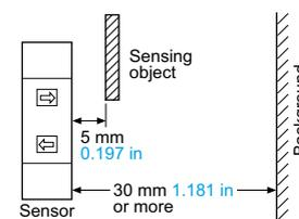
(However, the specular background should be a plane surface, directly facing the sensor. A spherical or curved background may be detected.)
