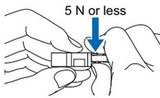
**Caution:** Be sure to hold a connector when plugging or unplugging it. Do not hold a terminal or a cable when plugging or unplugging the connector. Otherwise, it will cause a poor contact.
