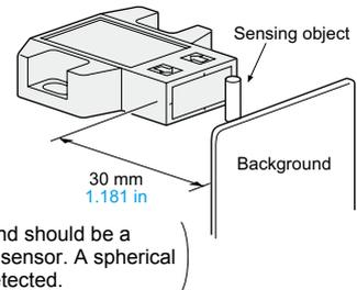
(However, the specular background should be a plane surface, directly facing the sensor. A spherical or curved background may be detected.)
