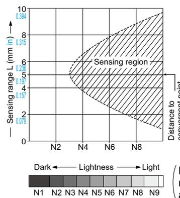
The sensing region (typical) is represented by oblique lines in the left figure. However, the sensitivity should be set with enough margin because of slight variation in products.
