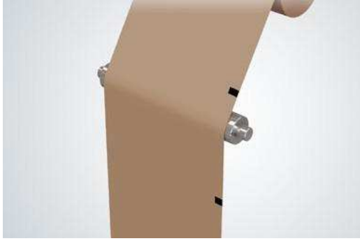
Registration mark detection on film
