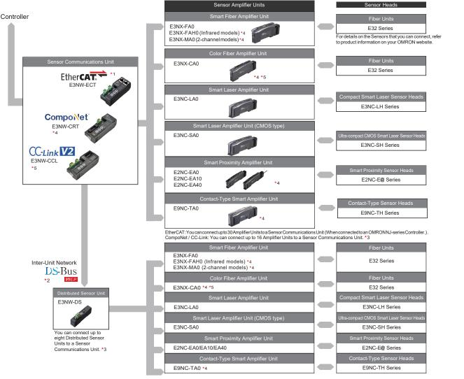
You can connect up to 10 Amplifier Units to a Distributed Sensor Unit. \*3
