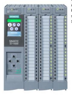
SIMATIC S7-1500 Compact CPU CPU 1512C-1 PN, central processing unit with working memory 250 KB for program and 1 MB for data, 32 digital inputs, 32 digital outputs, 5 analog inputs, 2 analog outputs, 6 high speed counters, 4 high speed outputs for PTO/PWM/frequency output 1. interface: PROFINET IRT with 2 port switch, 48 NS bit-performance, incl. front connector push-in, SIMATIC memory card necessary
