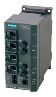
SCALANCE X204-2, managed IE switch, 4x 10/100 Mbit/s RJ45 ports, 2x 100 Mbit/s Multimode BFOC, LED diagnostics, error signaling contact with set button, redundant power supply, PROFINET IO device, network management; Redundancy Manager integrated, incl. electron. manual on CD-ROM, C-plug optional
