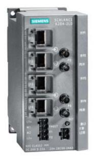
SCALANCE X204-2LD, managed IE switch, 4x 10/100 Mbit/s RJ45 ports, 2x 100 Mbit/s single-mode BFOC, Error signaling contact with set button, Redundant power supply, PROFINET IO device, network management, Redundancy Manager integrated, incl. electron. manual on CD-ROM, C-plug optional
