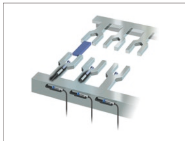
Confirming that a target is in transfer press grips
