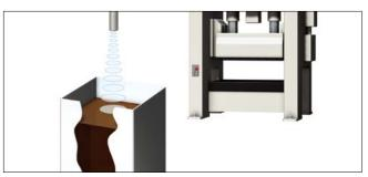
Detecting the liquid level of hydraulic fluid for a press Dirty oil has been difficult to detect with conventional contact liquid level sensors. The FW Series enables non-contact detection reducing the need for costly maintenance services.
