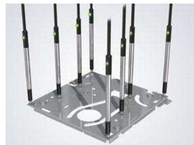
Chassis frame warpage inspection
