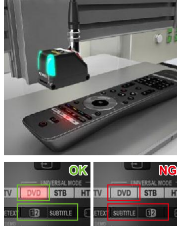
Remote control lighting check
