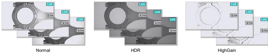
The optimal brightness is found automatically from multiple photographs taken under different image capture conditions.
