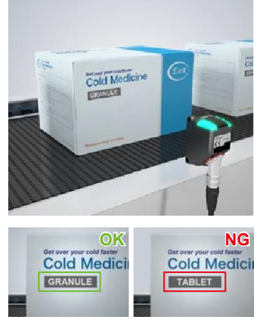
Product type detection according to text differences
