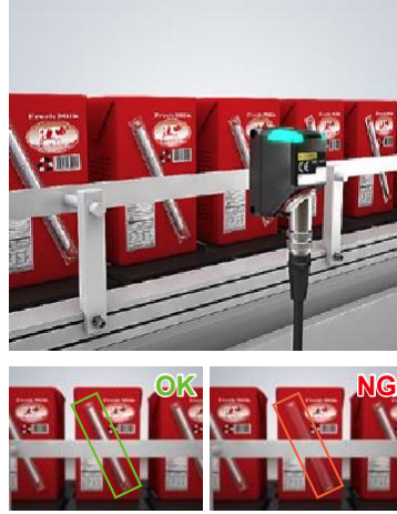
Missing straw detection
