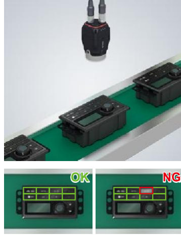
Button assembly defect detection
