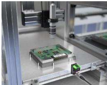
Connector pin breakage check
